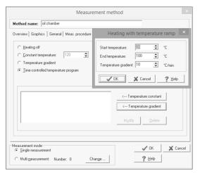
Preparation of measurement with temperature ramp
